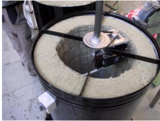
Insulated tube for motordriven turbine. Turbine hat taken off for looking inside.
